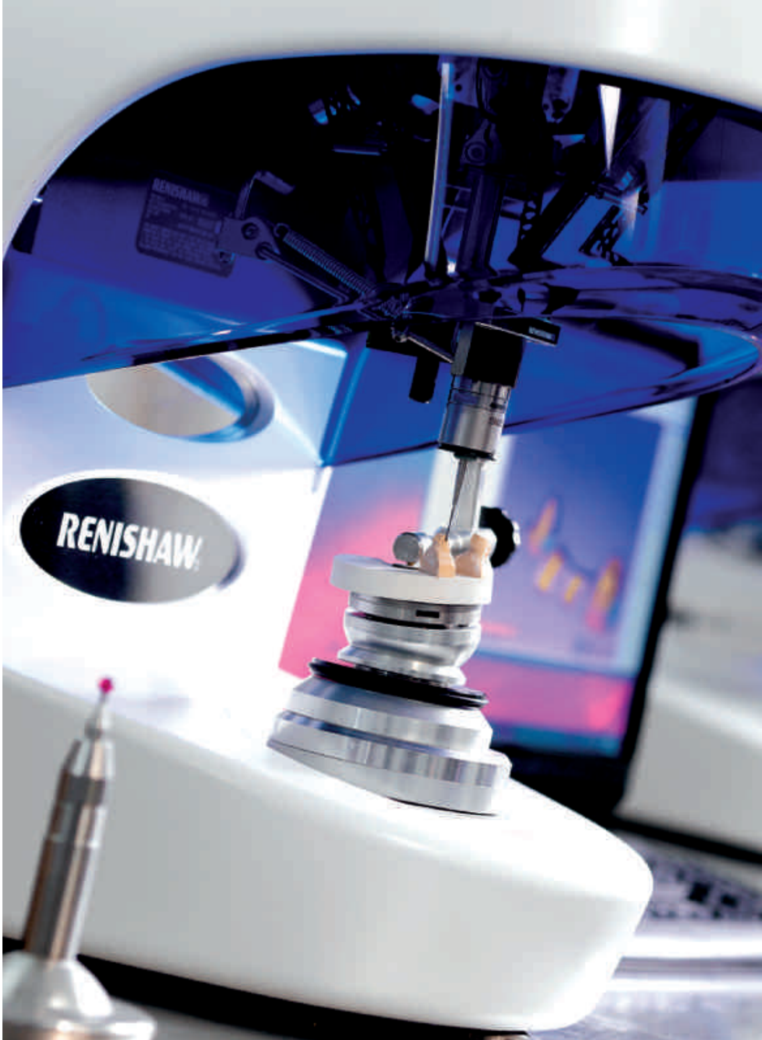
A Renishaw high-speed contact dental scanner in use at H2W, a UK dental laboratory, where it is used in the manufacture of high-quality zirconia dental frameworks.
