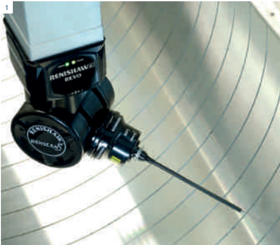
1: The REVO dynamic measuring head and probe system maximises the throughput of CMMs by providing greater accuracy, faster measurement, more automation and new capabilities. At Future Advanced Manufacture it has reduced measurement times on this high-precision imaging drum from one hour to just 10 minutes.
