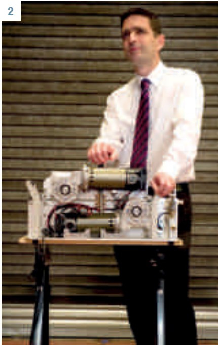
2: Nitzan Gonen, Factair's Design and Development Director, pictured with the patented portable 'fibre-blowing' machine that his company makes for a leading telecommunications company.
