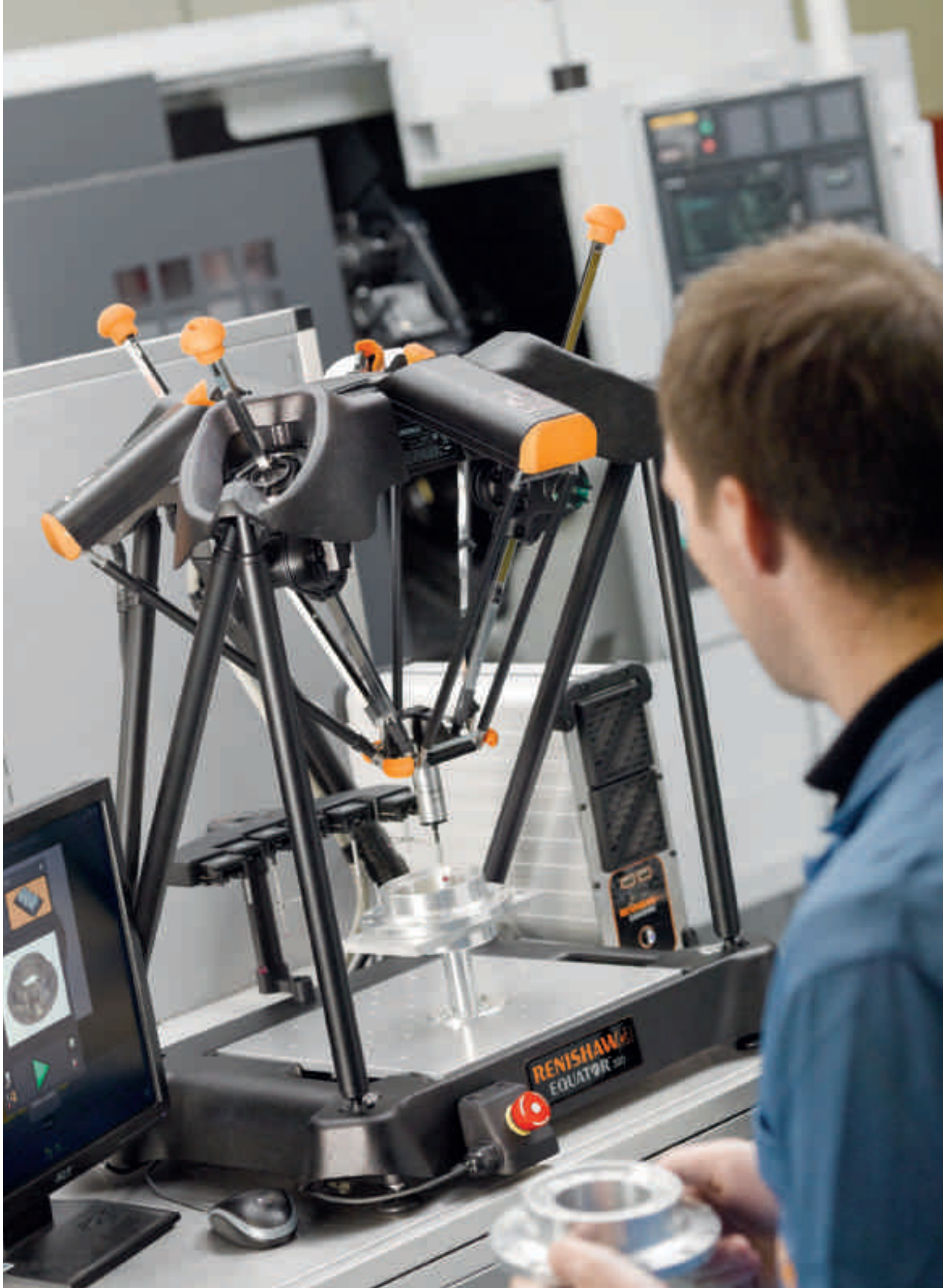
The new Renishaw Equator™ is a low-cost, versatile alternative to custom gauging, offering inspection of an unprecedented variety of manufactured parts. It has been developed and proven on the shop floor in collaboration with industry-leading companies in multiple industries and applications.
