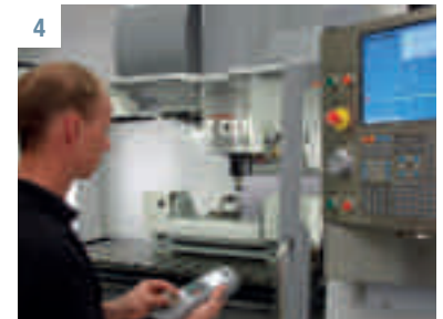
4: Introduced at the end of 2009, the QC20-W wireless ballbar is allowing manufacturers to rapidly assess the volumetric performance of their machine tools, without compromising safe working practices.
