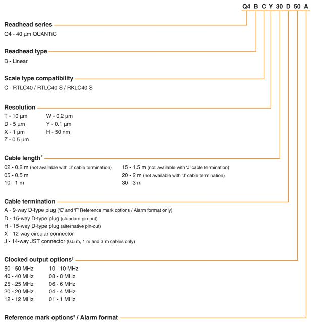
A - Customer selectable reference mark / Line driven alarm (not available with 'A' cable termination)
