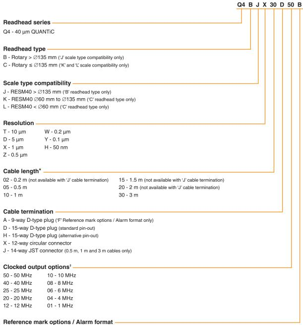
B - All reference marks are output / Line driven alarm (not available with 'A' cable termination)
