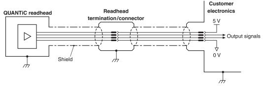
**IMPORTANT:** The shield should be connected to the machine earth (Field Ground). For JST variants the ferrule should be connected to the machine earth.
