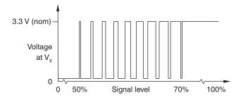
Between 50% and 70% signal level,  $V_{\rm x}$  is a duty cycle. Time spent at 3.3 V increases with incremental signal level. At > 70% signal level  $V_{\rm x}$  is nominal 3.3 V.
