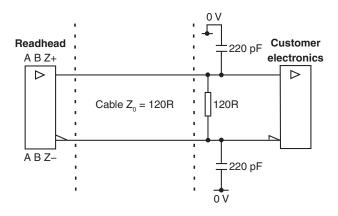
**Single ended alarm signal termination** (Not available with 'A' cable termination)
